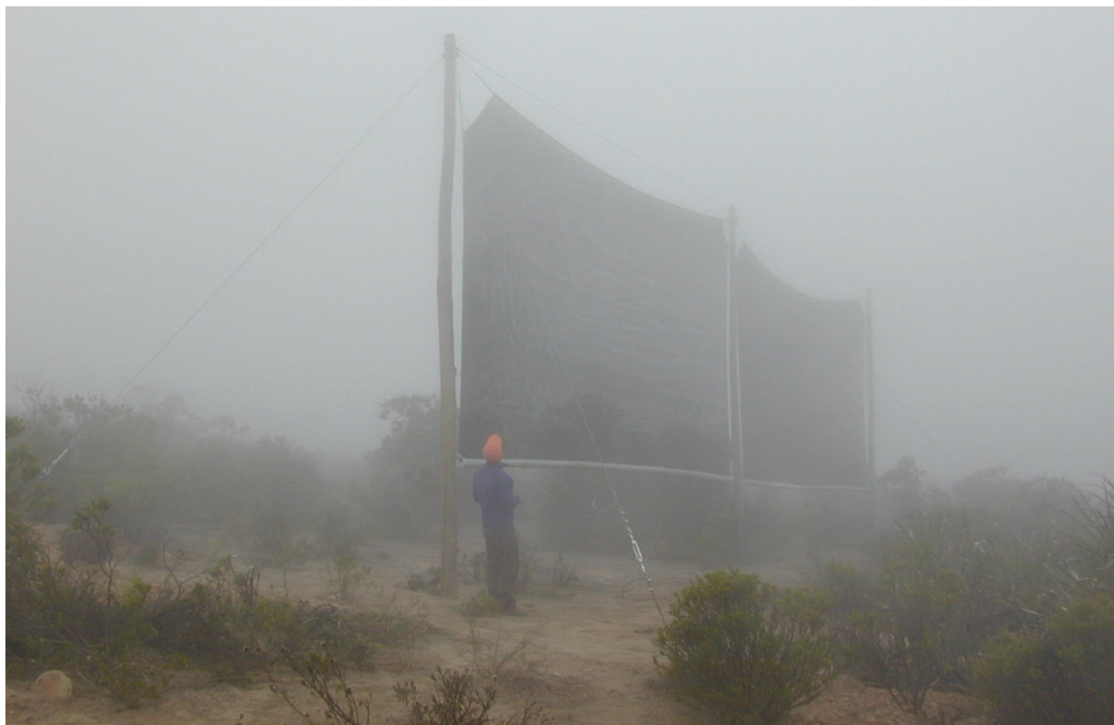
Figure 3. Large-scale fog collectors generate water when visibility is below 300 mm (Chile). Photograph: R. Schemenauer.
